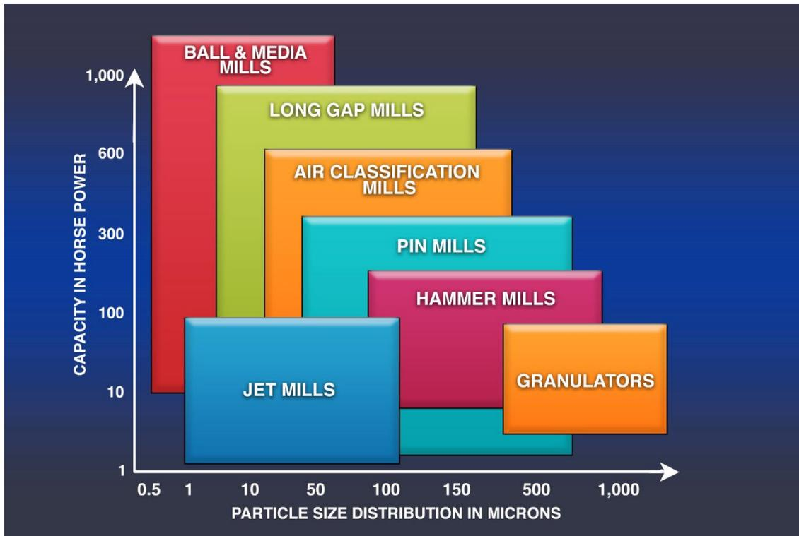
Figure 2: Particle size achievable by different types of mills designs. Source: [https://www.hmicronpowder.com/applications/size-reduction/?\\_vsrefdom=googleads&qclid=Cj0KCQiA95aRBhCsARIsAC2xvfwbZ3Dt48q6GXcONVkJQtTQVvKXYBU6ubsi5a7qba-HZr33wIY3GIDUaAISeEALw\\_wcB](https://www.hmicronpowder.com/applications/size-reduction/?_vsrefdom=googleads&qclid=Cj0KCQiA95aRBhCsARIsAC2xvfwbZ3Dt48q6GXcONVkJQtTQVvKXYBU6ubsi5a7qba-HZr33wIY3GIDUaAISeEALw_wcB)
