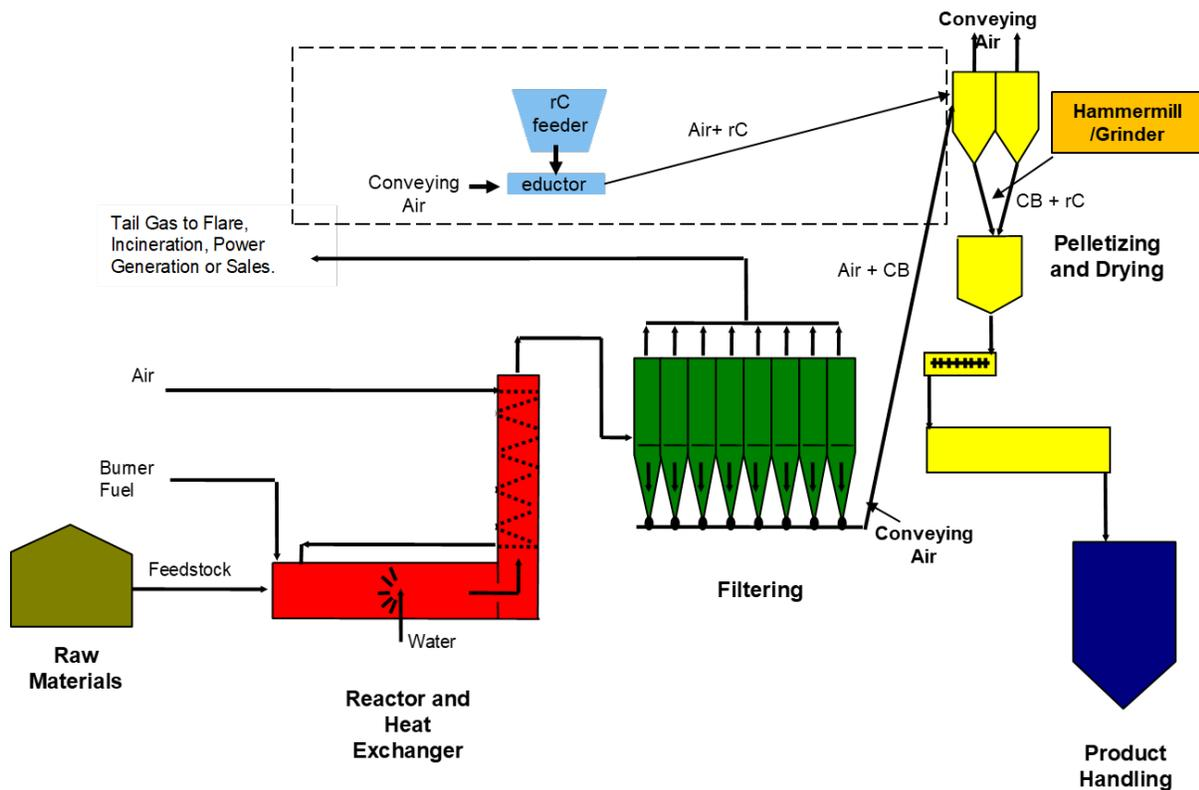
Figure 1: Schematic of Carbon Black production process with rC addition location
