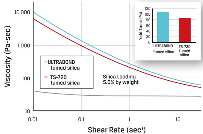
Cabot offers a range of highly hydrophobic, PDMS-treated silicas for rheology control of 1K PU adhesives. Of these, CAB-O-SIL ULTRABOND fumed silica provides the greatest increase in viscosity and sag resistance as predicted by yield stress.
