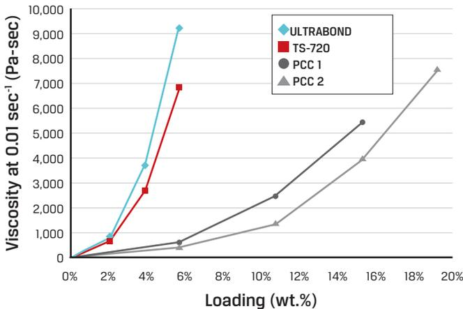
While coated Precipitated Calcium Carbonates (PCC) do increase viscosity and impart thixotropy in 1K PU adhesives, PDMS-treated fumed silicas are more efficient. Using a PDMS-treated fumed silica can provide sag resistance and rheology control without the significant weight (specific gravity) increase encountered with use of coated PCCs.
