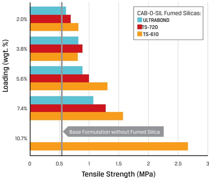
The addition of even low loadings of fumed silica will increase the tensile strength. At higher loading levels, CAB-O-SIL TS-610 DiMeDi treated silica provides greater reinforcement than the PDMS treated silicas.
