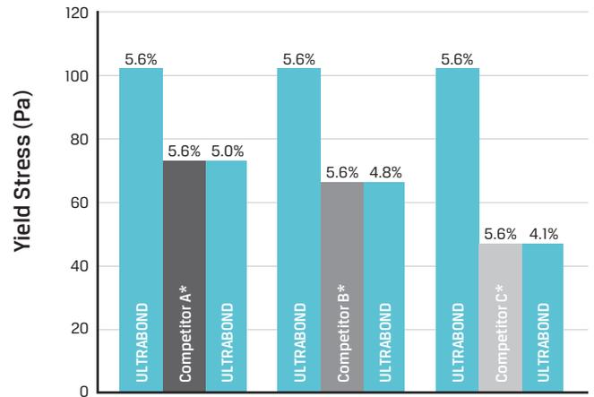
ULTRABOND fumed silica is one of the best thixotropes on the market for 1K PU adhesives. With ULTRABOND fumed silica, significantly lower loadings are required to achieve excellent sag resistance when compared with competitive PDMS-treated silica.
