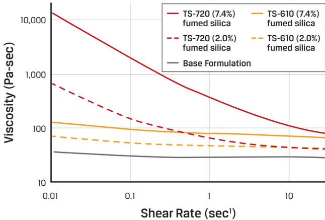
Silica surface treatment strongly influences rheological performance. Selecting a highly hydrophobic silica, such as CAB-O-SIL TS-720 fumed silica, imparts thixotropic or shear-thinning behavior in one-component polyurethane adhesives. In contrast, a moderately hydrophobic silica, such as CAB-O-SIL TS-610 fumed silica, imparts small increases in viscosity without thixotropy or shear-thinning behavior, even at increased loadings.
