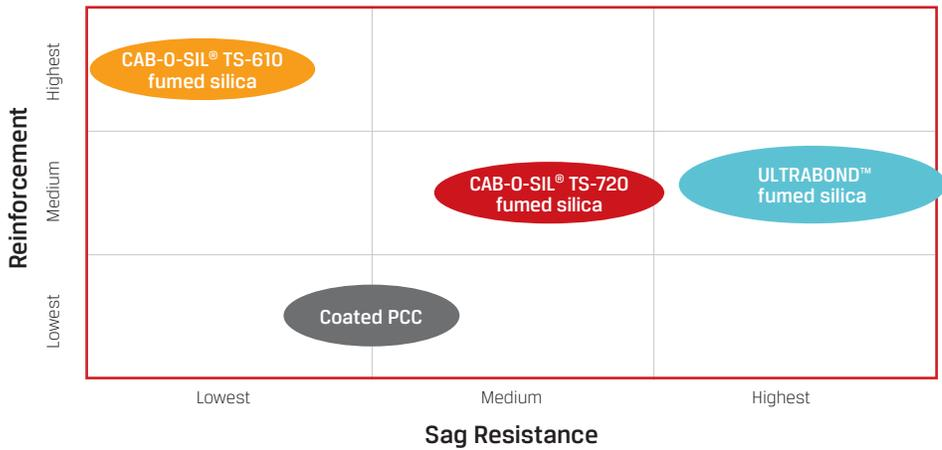
Cabot's portfolio of treated fumed silicas for use in 1K PU adhesives enables the formulator to readily optimize:
