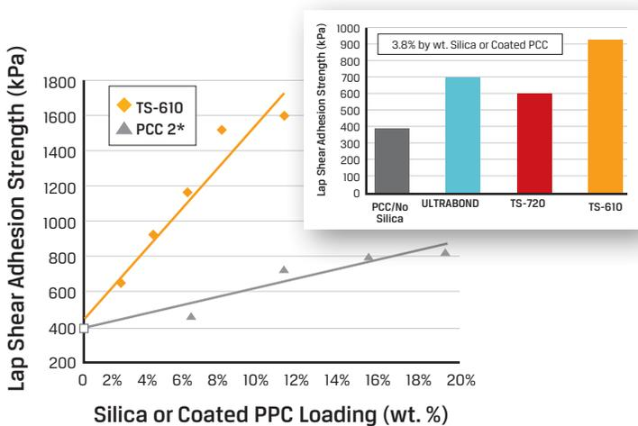
Coated Precipitated Calcium Carbonate (PCC) has only a modest effect on Lap Shear Adhesion Strength, while fumed silica significantly increases this strength.
