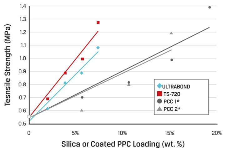
While both coated Precipitated Calcium Carbonate (PCC) and treated fumed silica can provide thixotropy, enabling formulation of sag-resistant adhesives, coated PCC has only a modest impact on mechanical properties.
