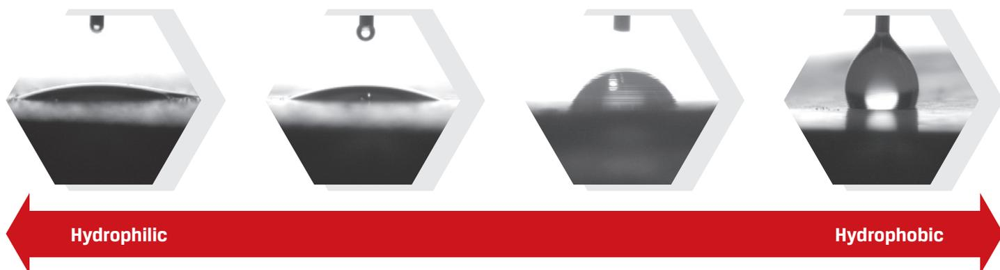
Figure 9: PBX carbon additives have surface properties ranging from hydrophilic to highly hydrophobic.
