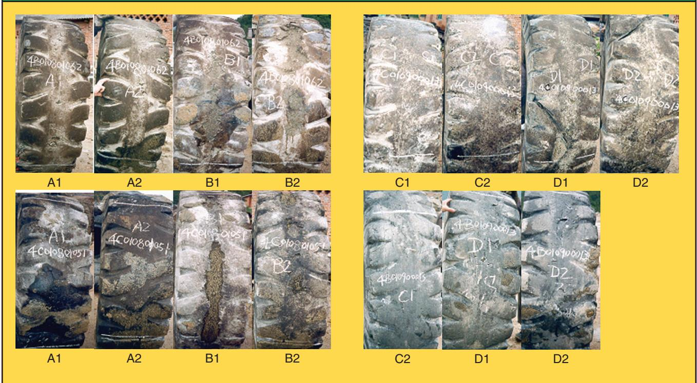
and then normalized the 1 pattern and 1/2 pattern to 1/4 pattern. From table 6 we can see that the NR compounds were better than the blend compounds in cut-and-chip resistance, and CEC compounds were better than the correspondent conventional compounds.
