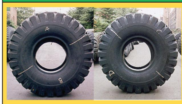
dexes from 22 tires. These are calculated and listed in table 5. Taking CEC counterparts as the reference, we can see that CEC material improved wear resistance at least 16% in the NR formulation and 12% in the blend formulation. Given that the CEC tread sections remained fully intact, it is evident that these wear resistance indexes are highly conservative, and that actual tire service life using the CEC material would have been longer.
